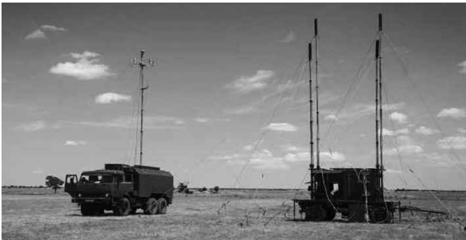
Fig 7: Russian R-330Zh Zhitel EW System
